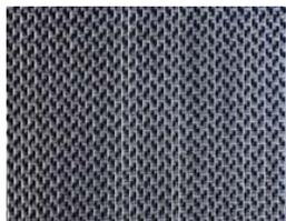
**Figure 3. Close-up view of a woven geotextile fabric. (Illustration image provided courtesy of Amoco Fabrics and Fibers Company, Atlanta, Georgia.)**
